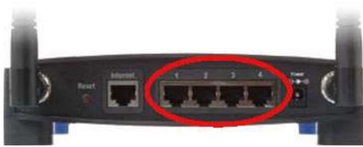
Fig. 2: Ethernet port sockets on the back of Linksys WRT54GL
