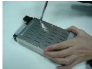
Step 4 Loose all screws on the Cartridge
