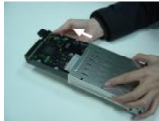
Step 5 Remove the HDD from Cartridge
