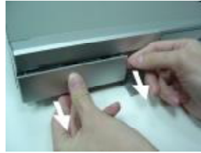
Step 3 Pull out the cartridge
